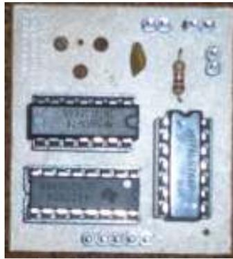
**Figura 3.8 – Interface Motor de Passo**
