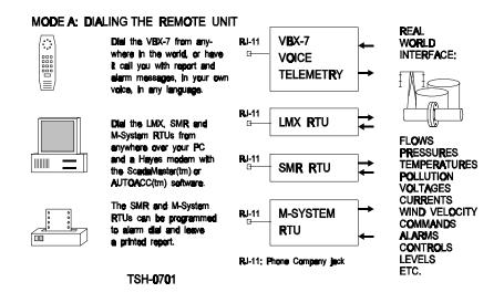
In many ways it works as if you placed a person instead of an RTU out at the remote site, a person you could call anytime, day and night. This person (or this RTU) answers the phone and tells you what is going on, the level of the tank, what pumps are on and off, what the pressure and temperature is, if there are any alarms, etc.
