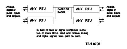
The Mode-C signal multiplexing systems use exactly the same continuous communication circuits as the Mode-B systems. The same considerations apply. Refer to section 7.G.1 above.
