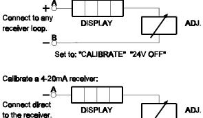
Calibrate any PLC, telemetry or other 4-20 mA input:
