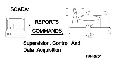
stopped), the flow rates and pressures, etc., are all now depicted in color graphics on your PC screen. You can start and stop any pump, for instance, by simply moving the cursor over to the 'START' or 'STOP' positions and pressing 'ENTER'. These supervisory systems are very capable and can automatically do a number of complex operations such as writing reports to a printer and/or to a disk drive, performing automatic control and alarm functions, etc.
