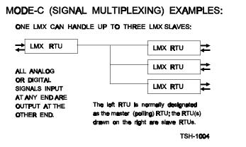
The M-system RTU will transmit and receive up to 4,000 points. To specify your M-system, simply add the I/O boards you need. All ScanData RTUs operate equally well over cable or radio, with their built in Bell-202 modems.
