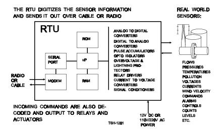
The RTU also receives commands over the radio and cable networks from a central or from another RTU to generate real world analog, digital and pulse current outputs. These commands are received in digitized form and are converted by the RTU to currents matching the requirements of the field relays, actuators and controller inputs.
