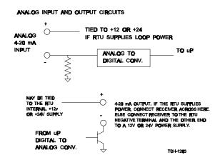
This class of outputs is almost always in the 4-20 mA form. This output current is used to drive motorized valve positioners, PLC setpoint inputs, meters, chart recorders and other process control devices.
