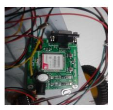
Figure 8 GSM SIM-900A Module
